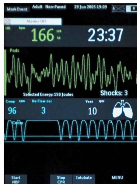
and then displayed as lung volume and ventilation rate on-screen. Just above the compression wave, the ventilation indicator shows lung volume. The calculated ventilations-per-minute (vpm) value appears next to the lungs indicator.
